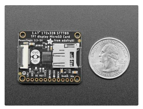
Note that the way we get the rounded corners is by deleting pixels. The corner pixels are still addressed in RAM, they just don't appear, so it isn't like you have to do some special radial-pixel mapping. Treat it like a rectangular display.
