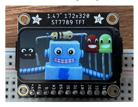
To make new bitmaps, make sure they are no bigger than the display size in pixels and save them in 24-bit BMP format! They must be in 24-bit format, even if they are not 24-bit color as that is the easiest format for the Arduino. You can rotate images using the setRotation() procedure
